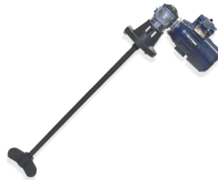
MIXN/8 Slow speed mixer 70/200 RPM. AISI shaft-PVC coated, different lengths available (630-730-830-930 mm). 3-blade impeller, diameter 150mm.
