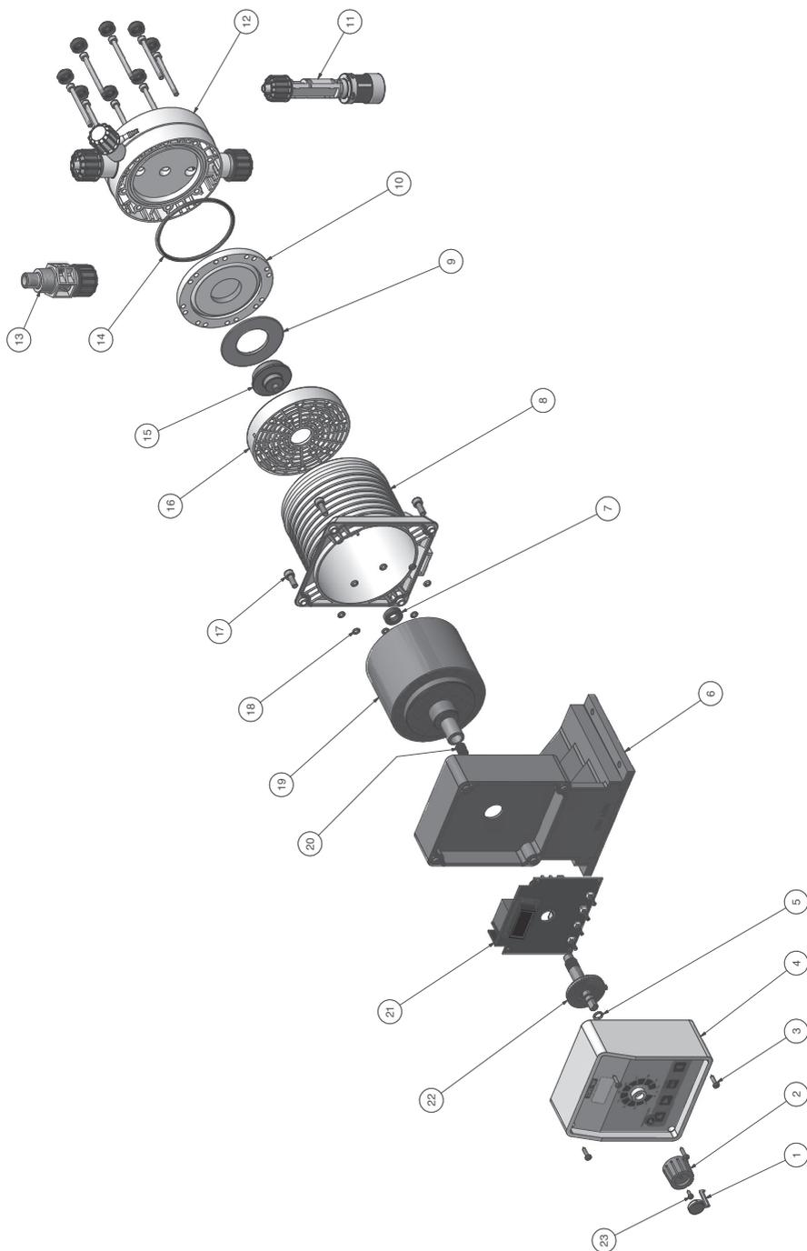
Fig. 53. Desenho explodido bomba AMSA MF
