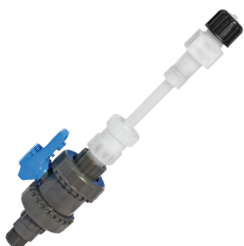
LINIR 1/2" injection lance for dosing sodium hypochlorite in hard water. Self cleaning. FKM B o-ring. PVC body.
