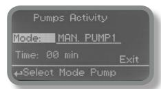
Exit from main menu. Main display will show a countdown including the selected pump (left for pH pump, right for Oxygen pump). To stop this countdown go back to "Pumps activity" menu and choose "ON" as working mode or wait until countdown ends. **This function can be used for priming purposes.**
