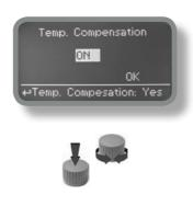
Instrument has either fixed or adjustable automatic temperature compensation referenced to a standard temperature of 25°C.
