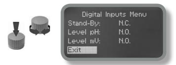
To end procedure move cursor on "OK" and press wheel to proceed to "Save" request screen. Move wheel on "YES" to save or "NO" to discard changes.
