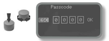
To set a new passcode choose "PARAMETERS" from "Main Menu", move on "New Pcode", click on wheel and enter a four numbers code. Click on "EXIT" and choose "YES" to save request. The new passcode is now ready.
