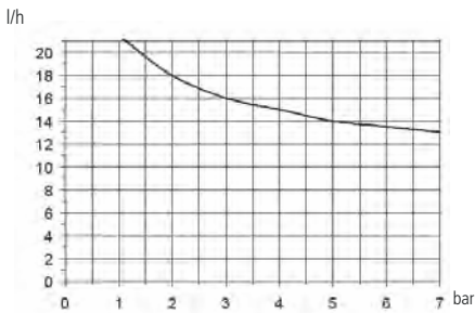
0713: l/h 13 bar 7 Pump head mod. NA
