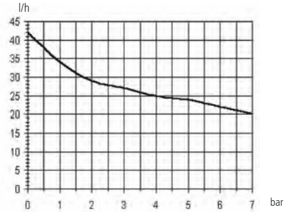
0720: l/h 20 bar 7 Pump head mod. N
