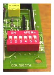
DIP 1: It enables conductivity alarm. Set it to ON to activate.
